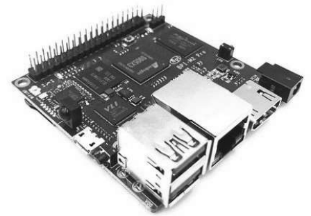
Banana Pi BPI-M2 Pro S905x3 design,same size and interface as BPI-M2+
