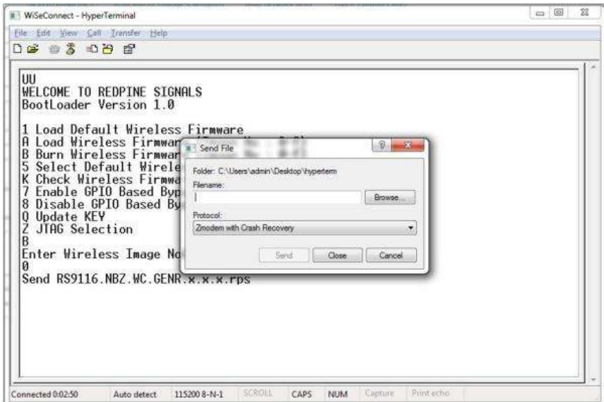
Figure 11: RYWB116 Module Firmware Upgrade File Selection Message
