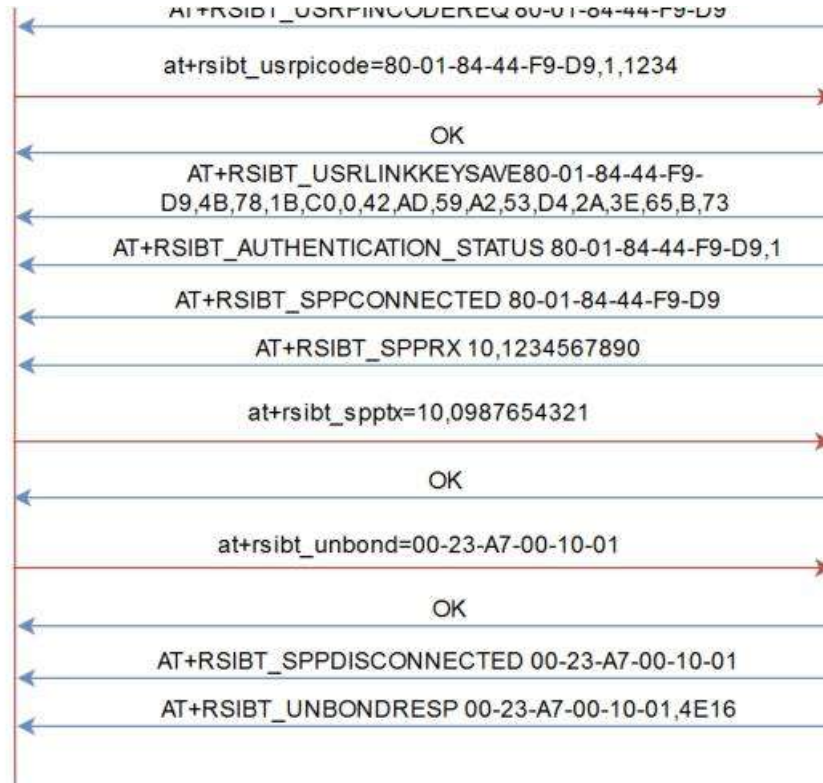
Figure 48: AT command flow in BT Slave mode
